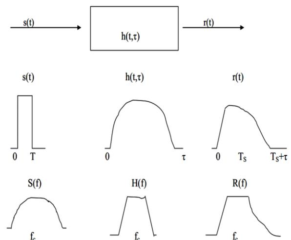
Fig. Frequency Selective Channel.
