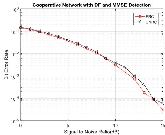
Figure 4.2 BER Vs SNR Curves using Relay Selection and MMSE Detection
