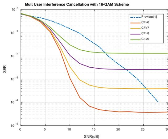
Fig.4.3 SER Performance of the OFDM System with different cancellation factors (CF) and 16-QAM Scheme
