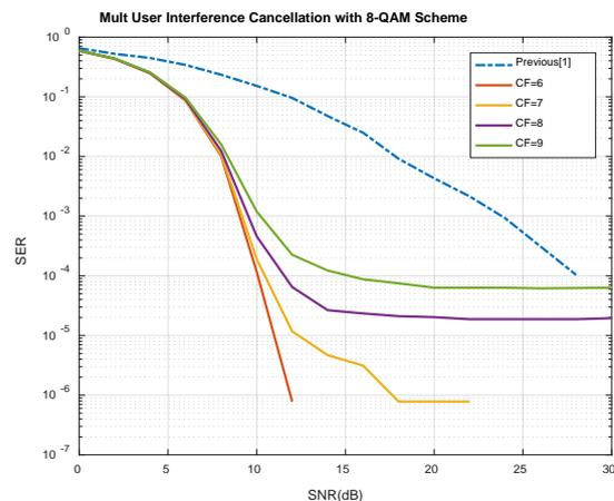
Fig.4.2 SER Performance of the OFDM System with different cancellation factors (CF) and 8-QAM Scheme
