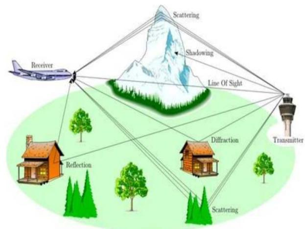
Fig.1.1 Multipath Propagation
