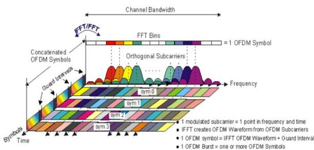
Fig.2.1 Frequency and time representation of OFDM spectrum
