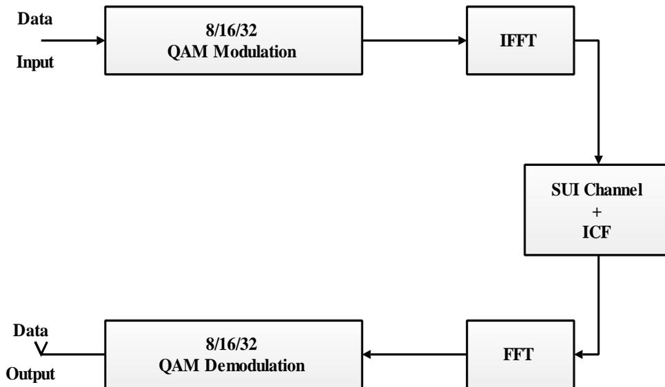
Fig.3.1 Block Diagram of Proposed System
