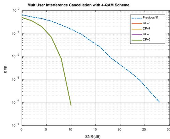
Fig.4.1 SER Performance of the OFDM System with different cancellation factors(CF) and 4-QAM Scheme
