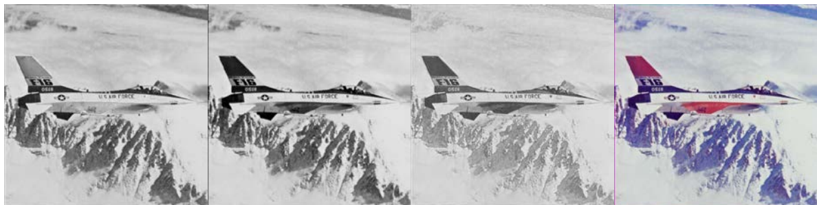
Fig.4.2 Compression Images: Red Layer, Green Layer, Blue Layer and Color Image of Plane Respectively.
