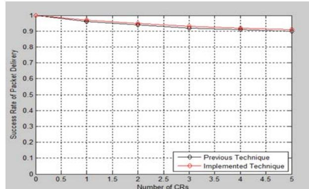
Figure 12: Number of CRs vs Success Rate of Packet Delivery
