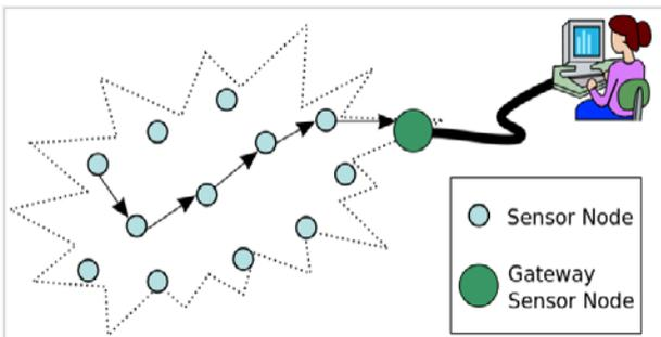
Figure 1: Typical multi-hop wireless sensor network architecture
