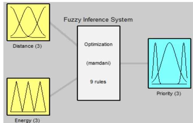
Figure 3: System Optimization of 2 inputs, 1 outputs and 9 rules
