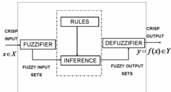
Figure 2. The structure of a fuzzy logic system
