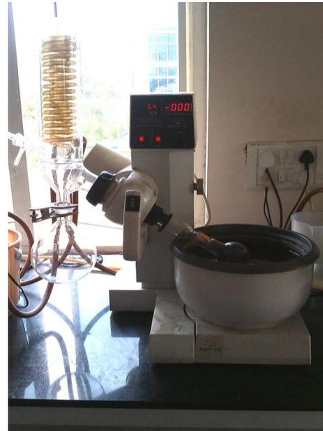
Fig 11: Rotary Evaporator
