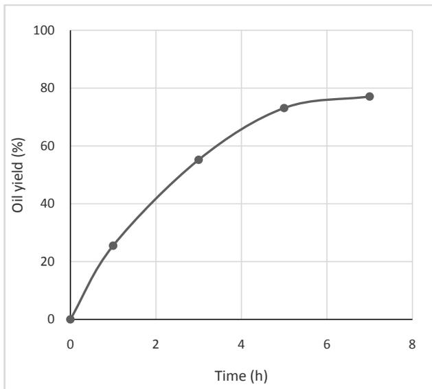
Fig 13: The reaction time was varied by keeping other parameters constant. The oil yield increased with the increase in the reaction time.
