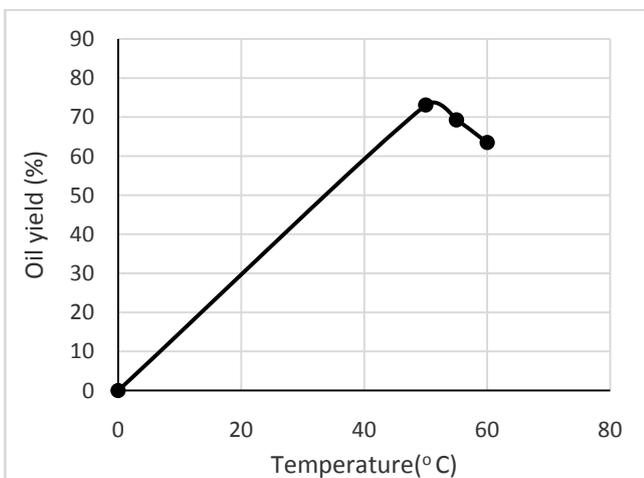
Fig 16: Effect of varying temperature on oil recovery by aqueous enzymatic oil extraction. The oil % obtained from the three different temperatures i.e., 50 °C, 55 °C, 60 °C
