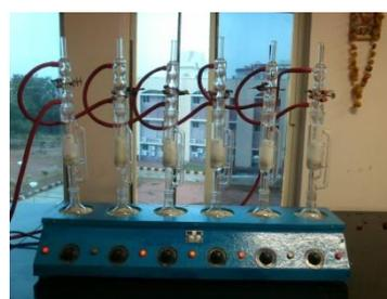
Fig 10: Soxhlet Extractor
