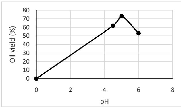
Fig 15: The aqueous oil extraction was done using 3 pH ranges i.e., 4.5, 5.0, 6.0. The results show that the enzyme activity is more at pH 5.0 therefore resulting in higher oil liberation.
