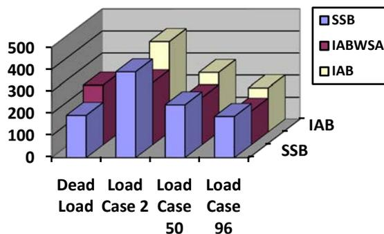
Chart 3: Stresses Developed in Top Deck Slab
