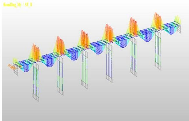
Fig 2 Integral Abutment Bridge Bending Moment diagram
