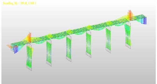
Fig 3 Integral Abutment Bridge (Spring Analysis at Both End Abutments Bending ) Moment Diagram (IAB WSA)
