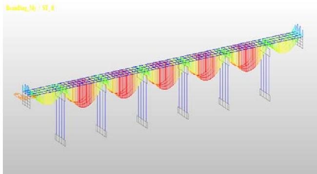
Fig 1 Simply Supported Bridge Bending Moment Diagram
