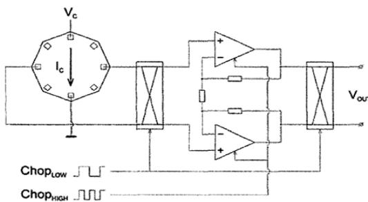
Figure 7. Schematic overview of the EMF measurement IC.
