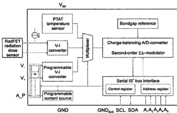
Figure 10. Block schematic overview of the space-qualified instrumentation ASIC
