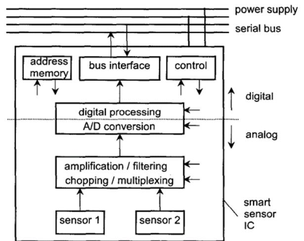
Figure 1. Basic functions in a smart sensor IC.
