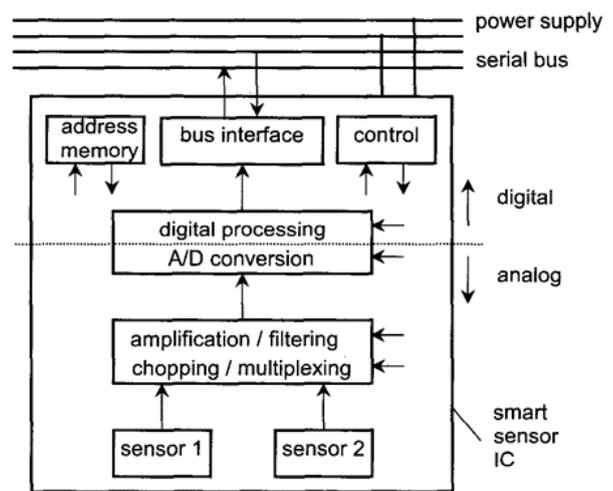
Figure 1. Basic functions in a smart sensor IC.
