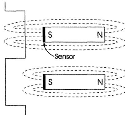
Figure 8. Magnetic-field variations caused by the presence of metal.
