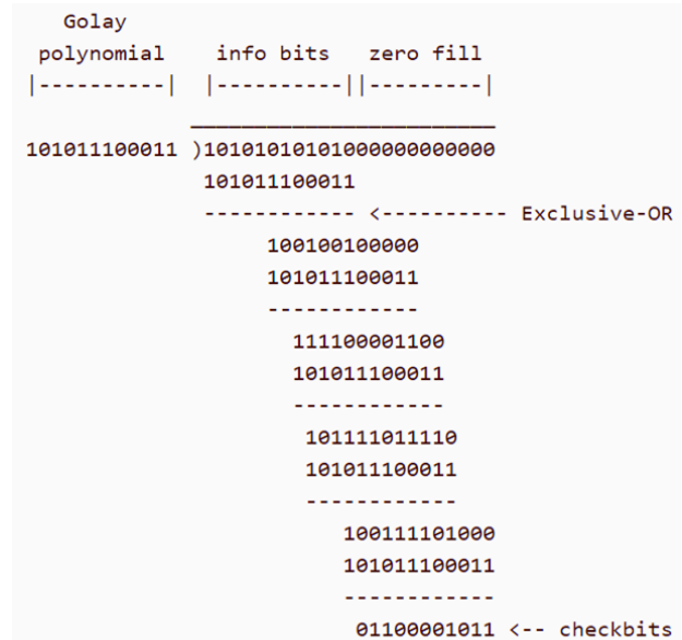
Figure 2: Golay Encoder Example
