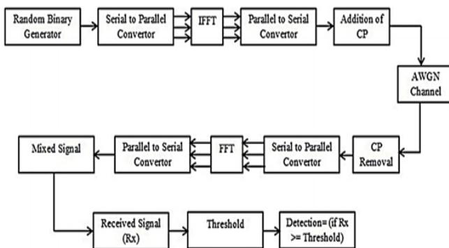
Figure 4: MIMO-OFDM System using Matched Filter Detection Technique
