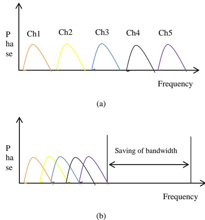
Figure 1: Comparison between conventional FDM (a) and OFDM (b)
