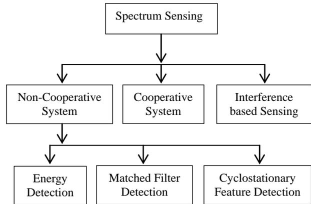
Figure 3: Classification of spectrum sensing techniques
