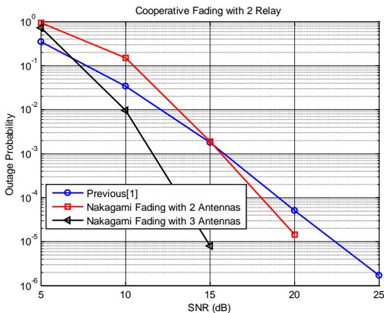
**Figure: 5.2 Outage Probability of Dual Hop Cooperative Relay system with multiple antennas and R=2.**
