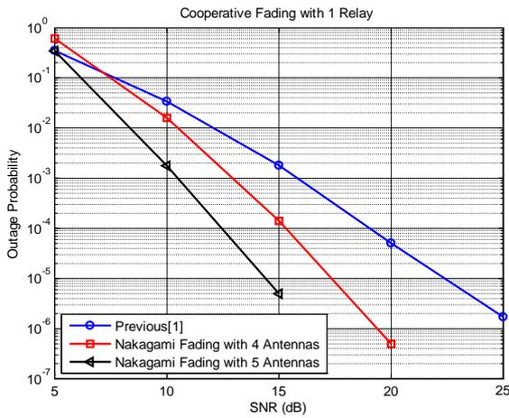
**Figure: 5.1 Outage Probability of Dual Hop Cooperative Relay system with multiple antennas and R=1.**
