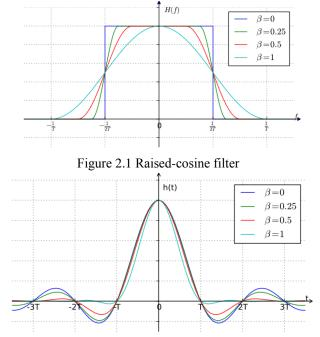
Figure 2.2 Impulse response of Smoothening Filter. Raised cosine window is utilized as a part of increased with window work. Raised cosine work is characterized as takes after where beta is move off factor expands side lobe of OFDM range decreases. This decrease inside lobe level ICI control prompts the diminishment in ICI.
