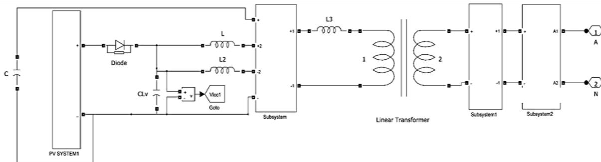
Figure. 3.2 PV System in Simulink.
