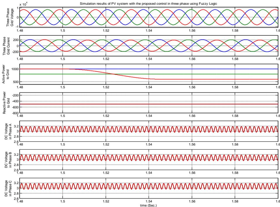
Fig. 4.2 Simulation Results of Proposed Decoupled Grid Connected PV System of Three Phases.
