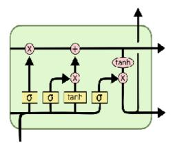
Fig 4.2: LSTM Architecture
