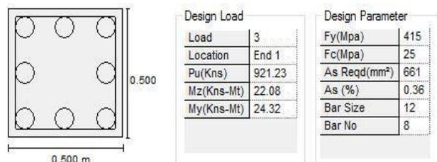
**Figure 8; Reinforcement details of column No.14 in STAAD Pro. Using design code IS- 456:2000**
