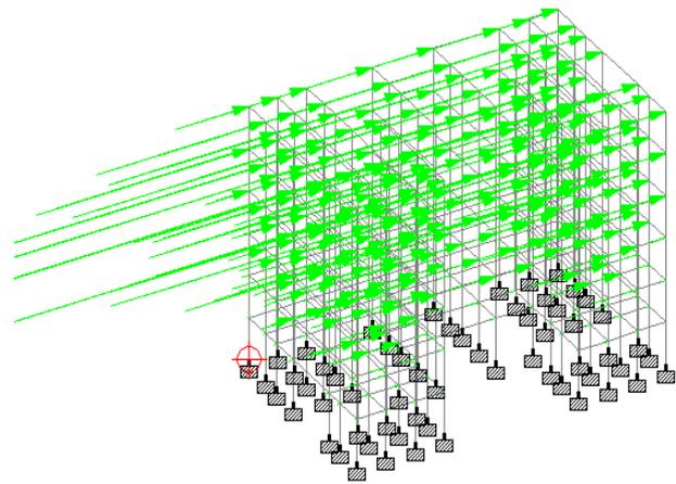
Figure 13 ; showing the seismic load acting from +x direction (Isometric view)
