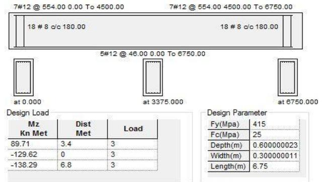
**Figure 5; Reinforcement details for beam No.412 in STAAD Pro. Using design code IS- 456:2000**
