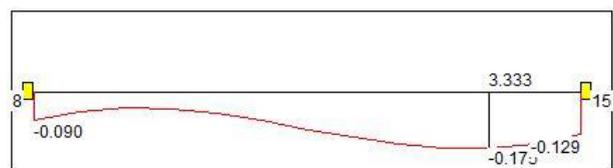
**Figure 7 ; Deflection diagram of column No. 14**
