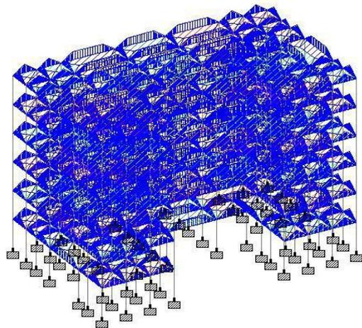
Figure 2; The live load acting on the structure
