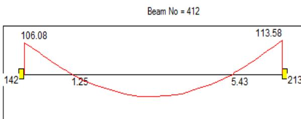
Figure 11; Bending moment due to seismic combination load
