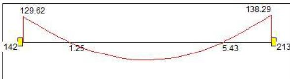
**Figure 3 ; Bending moment diagram of beam No.412**
