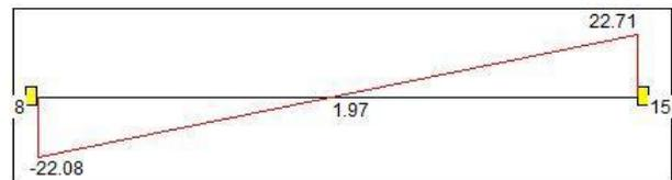
**Figure 6 ; Bending moment diagram of column No. 14**
