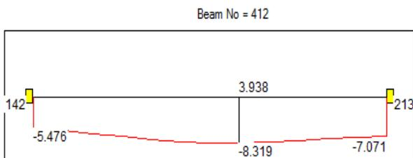
Figure 10 ; Beam deflection due to seismic combination load
