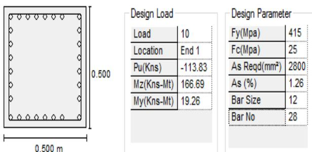
Figure 12; Shows the Column details due to Seismic Load Combination
