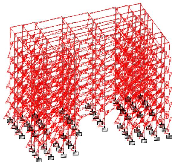
Figure 14; Bending moment diagram due to seismic force from +x direction
