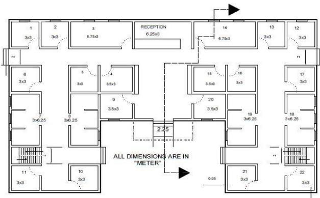
Figure 1; Plan of six- story RC building (all dimensions are in mm)
