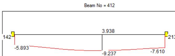
**Figure 4 ; Deflection diagram of beam No.412**
