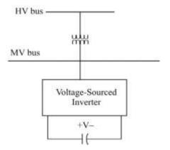
STATCOM is used to provide reactive power to the AC arrangement, alongside that, it will offer the DC power necessary for both inverters. The thoughtless power can be
