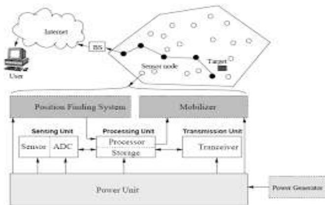
Figure 1: wireless sensor network with node architecture
