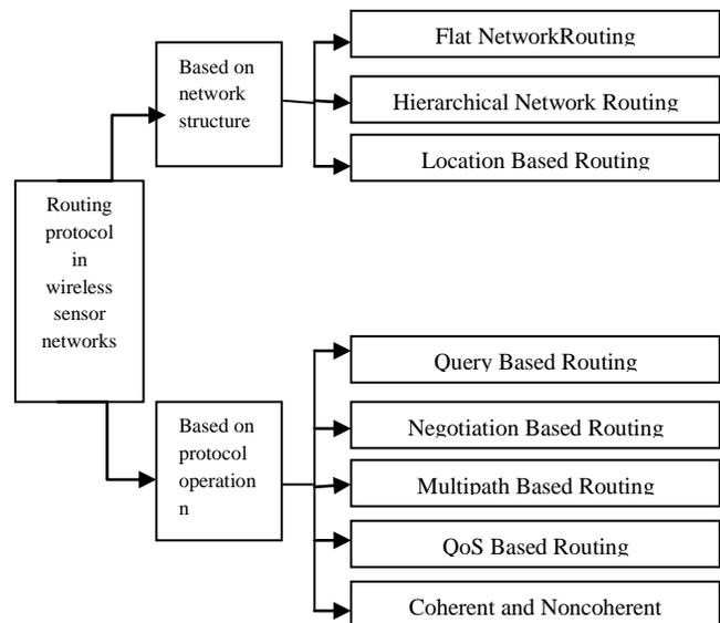
Figure 5: Routing Protocols in Wireless Sensor Network
