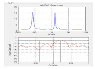
In this figure we display the simulation result of smart antenna using direction of arrival (DOA) estimation and MVDR algorithm for same angle with SNR=60 and N=7 elements.
