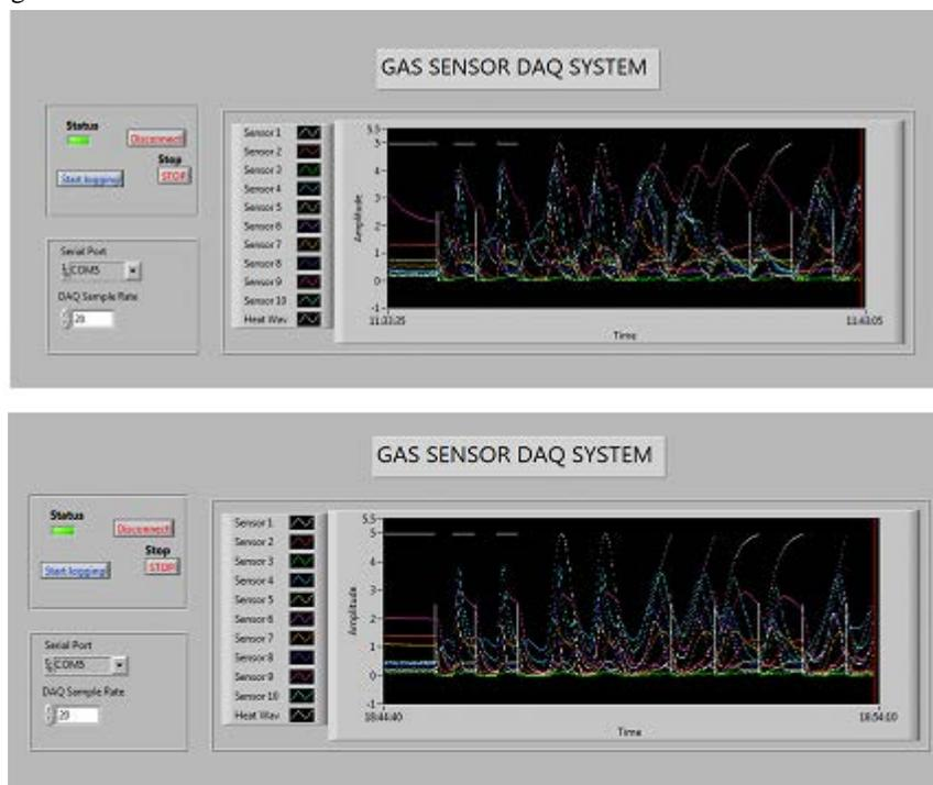
Fig 3.1: Response of gas sensors to acetone and butanol for six differently modulated heater voltages
