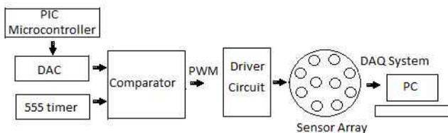
Fig. 2.1: Experimental data-acquisition setup
