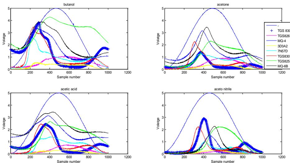
Fig 3.2: Response of the eight gas sensor to four different gases A) for sinusoidal heating waveform and B) for sigmoid heating waveform
